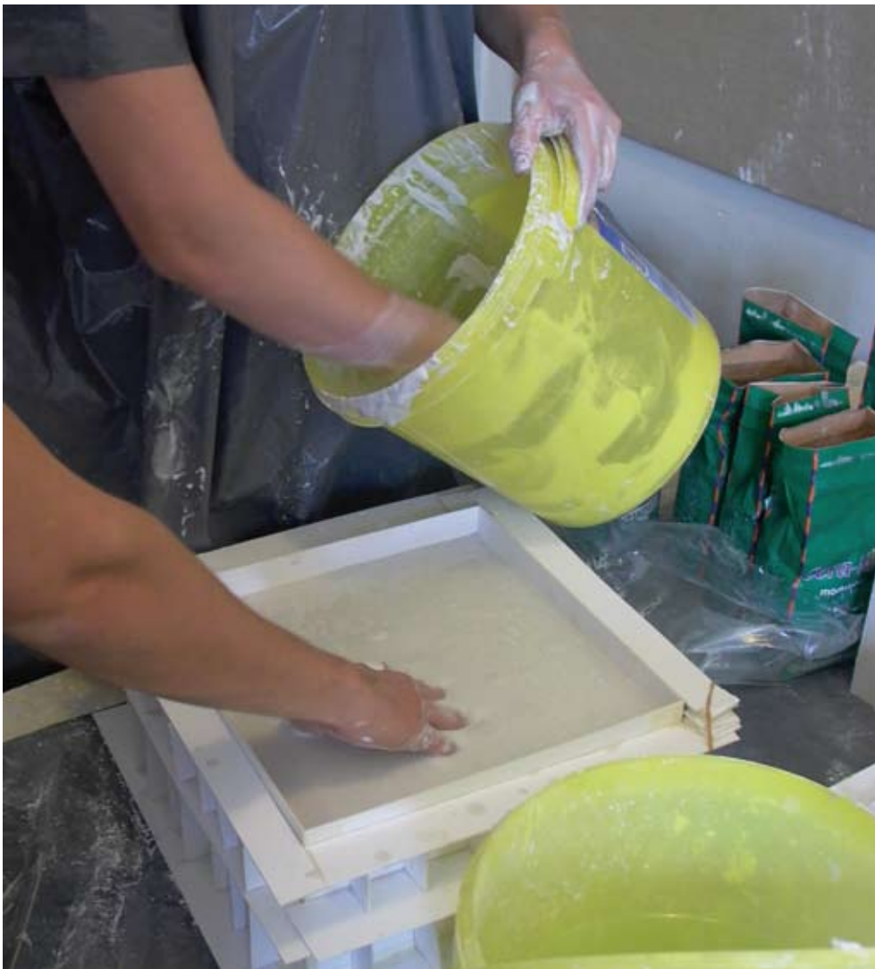
This page Casting the mould in plaster
